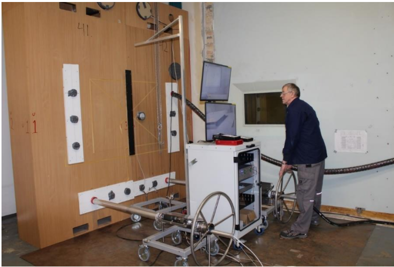
Figure 19: Operator testing the mock-up of a Hot Cell
