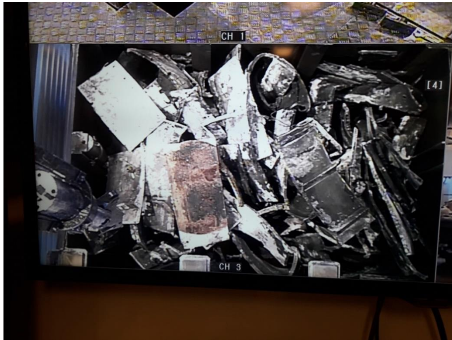
Figure 14: Lead sheets in the DD type 2 steel container
