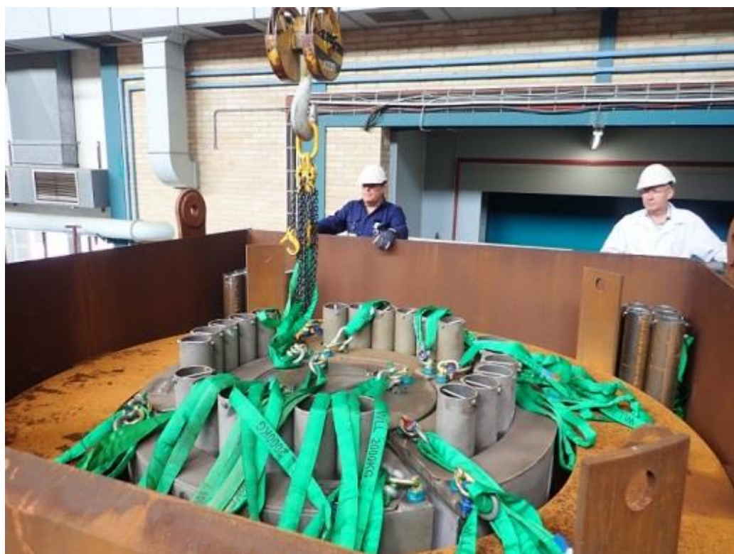
Figure 6: The centre of TSR is filled with the centre container surrounded by the four ¼ moon containers.
