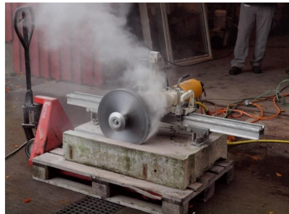
Figure 32: The milling tool in action
