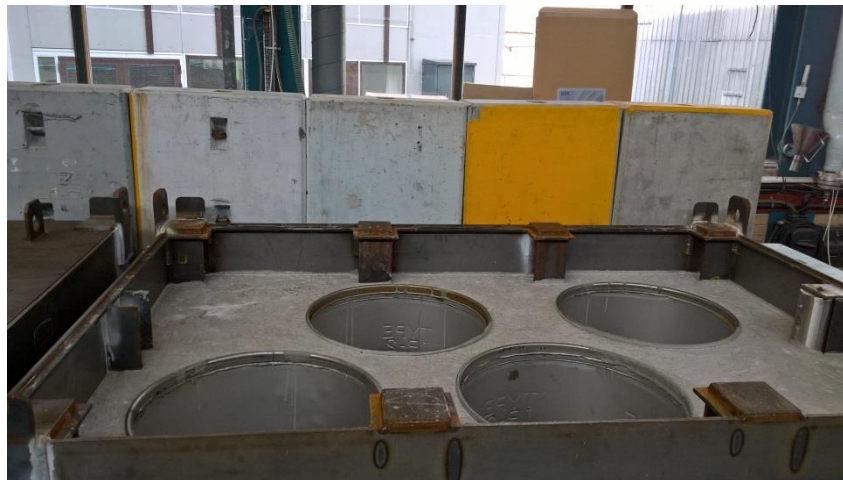
Figure 8: Four steel drums placed in a standard DD type 2 steel container back-filled with concrete
