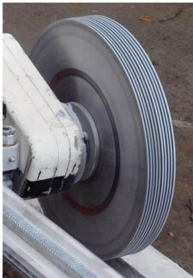
Figure 33: The closely spaced saw blades forming a milling tool capable of milling a 10 cm broad groove in the concrete
