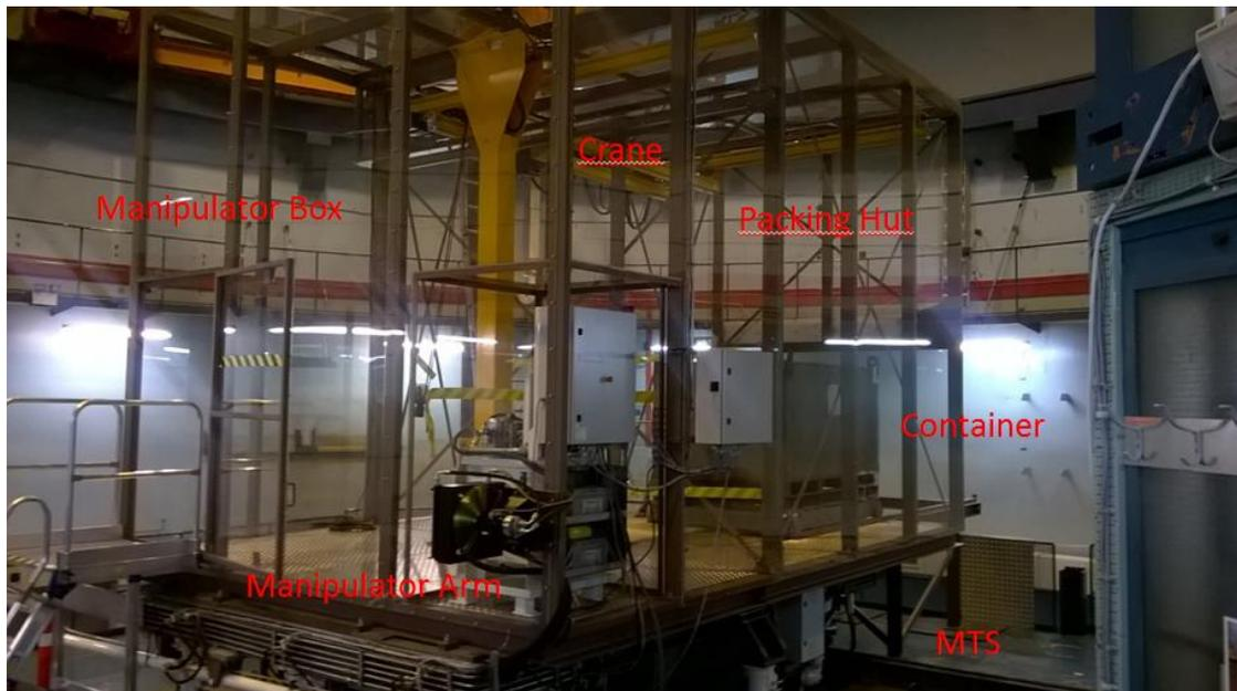
Figure 2: The Packing Hut and the Manipulator Box installed on the MTS on the reactor top.
