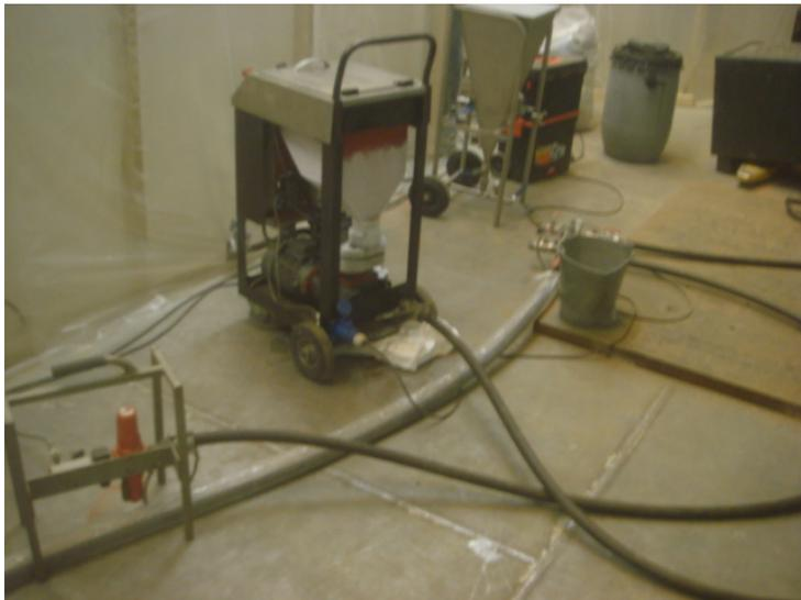
Figure 6: The CO<sub>2</sub> ice blasting equipment
