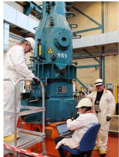
Figure 18: Flask for handling experimental rigs placed on a viewing box.
