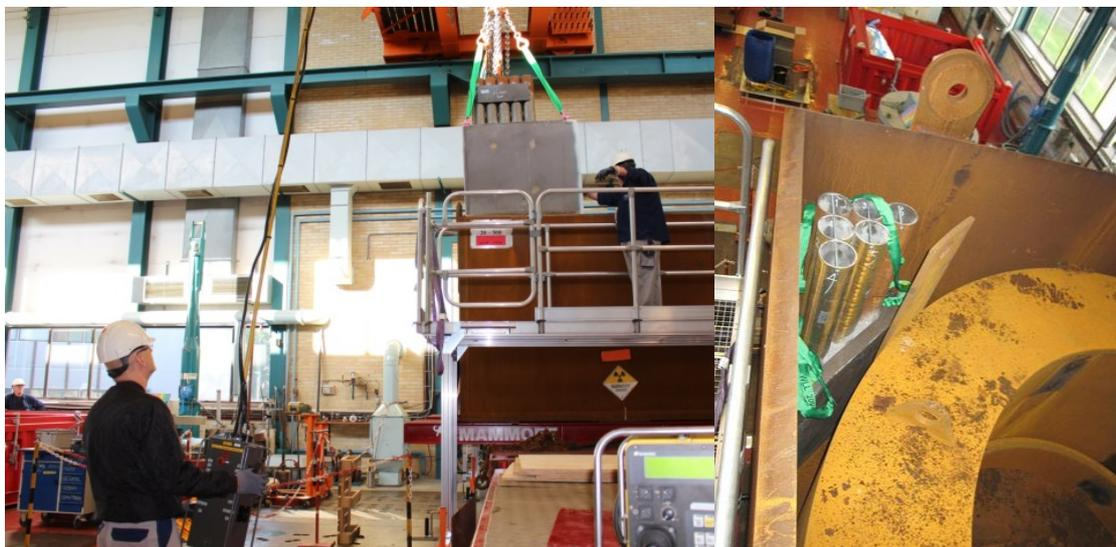
**Figure 12: Loading a corner container with FE-plugs into a Jumbo container.**
