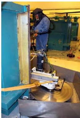
Figure 22: Circular saw for cutting the shutters.
